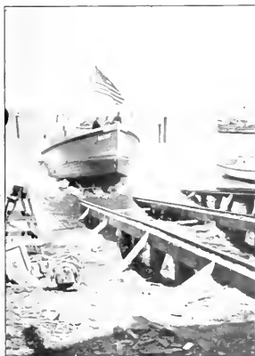
The new twin screw power boat Salana, sliding off the ways at the Anderson & Siemer yard, San Francisco. Note the flat bottom.
